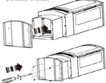
**4.** Secure the base to the pillar with the screws previously removed.
