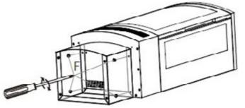
**3.** Secure the base to the pillar with the 4x screws previously removed.]
