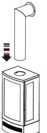
2. Using two (2) people, move the appliance to where you would like it to be installed. Insert the small end of the Flue Pipe into the top recessed hole on the appliance, also ensuring that the opposite flanged end of the pipe is touching the wall.
