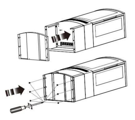
4. Secure the base to the pillar with the screws previously removed.
