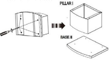
2. Lay the appliance on its back and assemble the Pillar on to the bottom of the appliance with the firebox provided screws (F)
