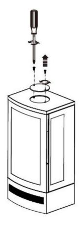
With a cross headed screw driver unscrew the two (2) countersunk head screws from the decorative grill plate on top of the appliance. Carefully leaver the decorative grill plate off of the top of the appliance through the screw holes.
